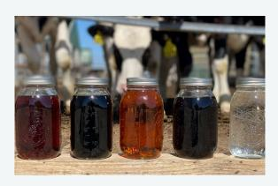
ZwitterCo superfiltration (permeate in the center) enables this treatment process by protecting the RO from small molecule, heavy foulants. The result is the consistent generation of a highly concentrated nutrient stream (second from the right) and a reusable or dischargeable clean water stream (far right).
