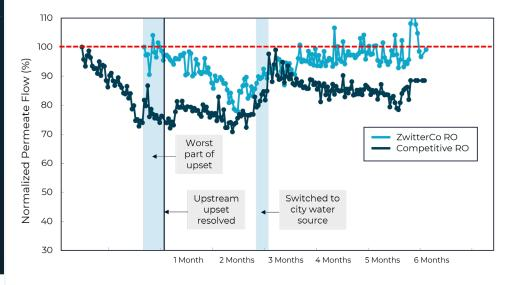
A United States-based power plant treating river water for boiler makeup was cleaning their two-train RO system once a month and replacing elements every 1-1.5 years due to persistent organic fouling challenges.
