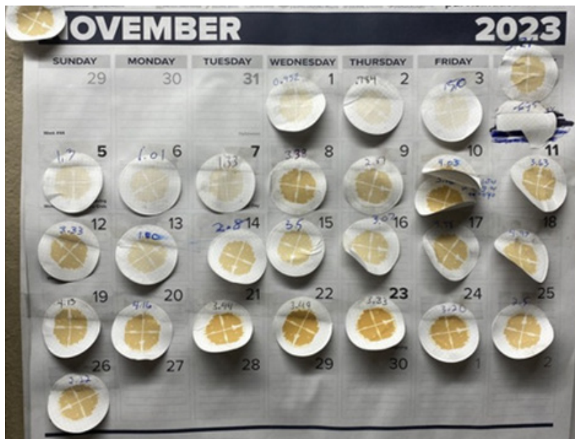
Figure 2: Coupons showing the SDI increase from a coagulant upset in November 2023, confirming higher contaminant levels in the RO feed.
